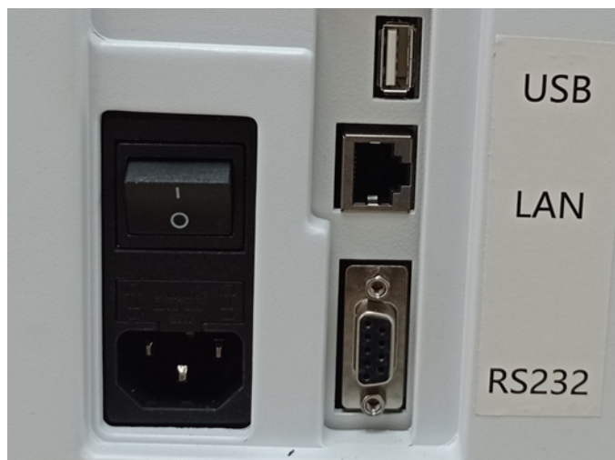
Figure: Power outlet location
